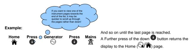
Once selected, the page will remain on the LCD display until the user selects a different page or, after an extended period of inactivity (*Page Delay Timer*), the module reverts to the Home () page.
