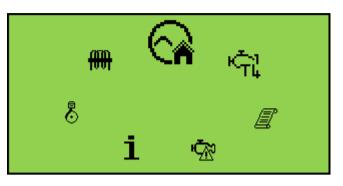
To select the required icon, press the • (up) button to cycle right or the • (down) button to cycle left until the desired instrumentation section is reached.
