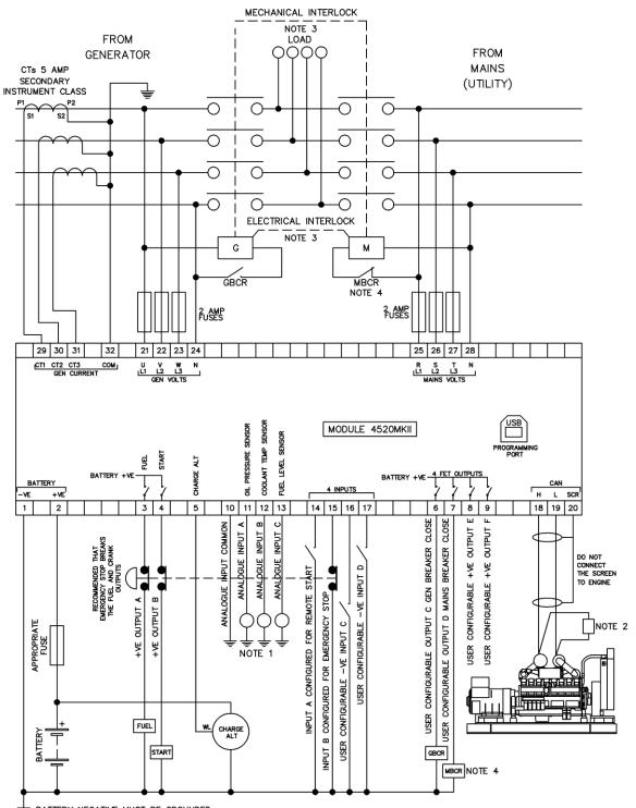
➡ BATTERY NEGATIVE MUST BE GROUNDED NOTE 1. THESE GROUND CONNECTIONS MUST BE ON THE ENGINE BLOCK, AND MUST BE TO THE SENSOR BODIES.
