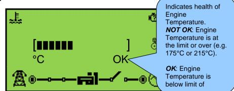
Engine Temperature has 2 different options for display mode the bars are not linear. The table below can be referenced for the Temperature represented in the bar graph.
