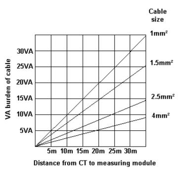
must be used. If 2.5 mm<sup>2</sup> cables are used over the same distance of 20 m, then the burden of the cable on the CT is approximately 7 VA. CT's required in this instance is at least 7.25 VA (7 + 0.25).
