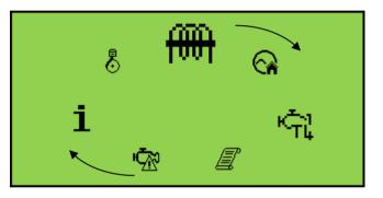
Once the desired icon is at the top, press the **Auto Mode**  $(\checkmark)$  button to enter that instrumentation section. If the **Auto Mode**  $(\checkmark)$  button is not pressed, the display automatically returns to the Home  $(\checkmark)$  page after the configured setting of the *LCD Scroll Timer*.
