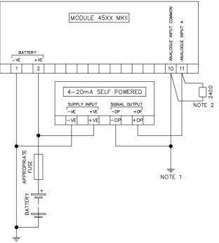
NOTE 1. THESE GROUND CONNECTIONS MUST BE ON THE ENGINE BLOCK, AND MUST BE TO THE SENSOR BODIES. NOTE 2. WHEN USING A 4–20mA SENSOR, AN EXTERNAL 240 $\Omega$  RESISTOR MUST BE FITTED ACROSS TERMINALS 10 AND 11.
