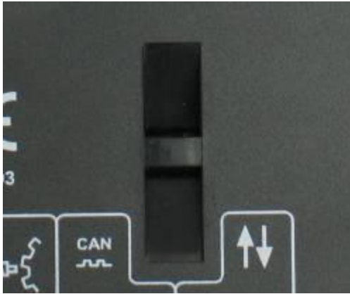
Cable Tie Fixing Point
