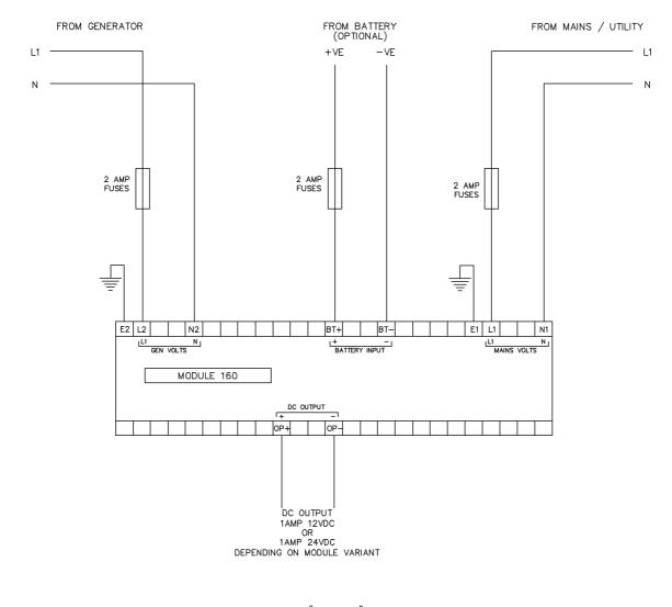
TERMINALS SUITABLE FOR 22-16 AWG  $(0.6mm^2 - 1.5mm^2)$  FIELD WIRING TIGHTENING TORQUE = 0.8Nm (71b-in)
